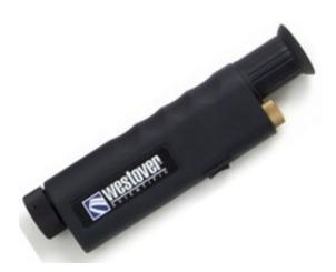
The 200X Dual illumination Optical Microscope is a dual illumination 200x microscope. It uses a pair of white LED's to provide both coaxial and oblique illumination. This lighting technique facilitates both detecting fine scratches and precisely determining their location relative to the core.
